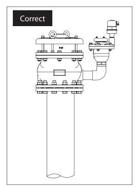
$\textbf{3.} \ \ \, \text{The standpipe should be attached to the crown of the pipe and not from the side of the pipe.}$
