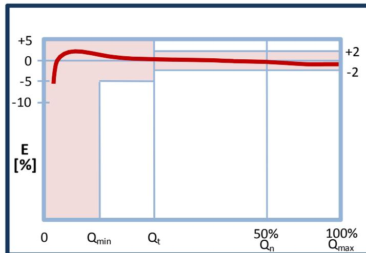
**Figure 1.1** Performance curve of a new water meter
