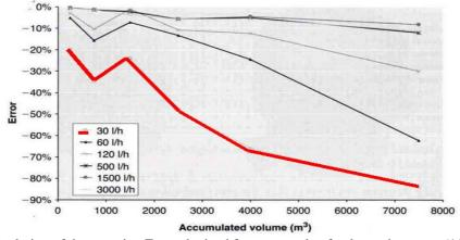
**Figure 3:** Evolution of the metering Error obtained from a sample of volumetric meters (1/2") (Arregui el. 2006, p.28)
