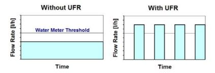
Figure 7: UFR – Principle of Operation
