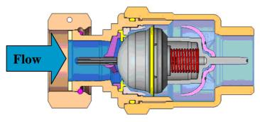
Figure 8: UFR closed: downstream pressure decreases because of leakage
