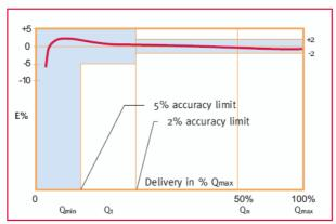
Figure 1: Error curve of a water meter
