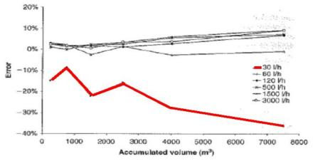
Figure 2: Multi-jet error (nominal flow 1.5 m<sup>3</sup>/hr) on accumulated volume (Arregui el. 2006, p.21)
