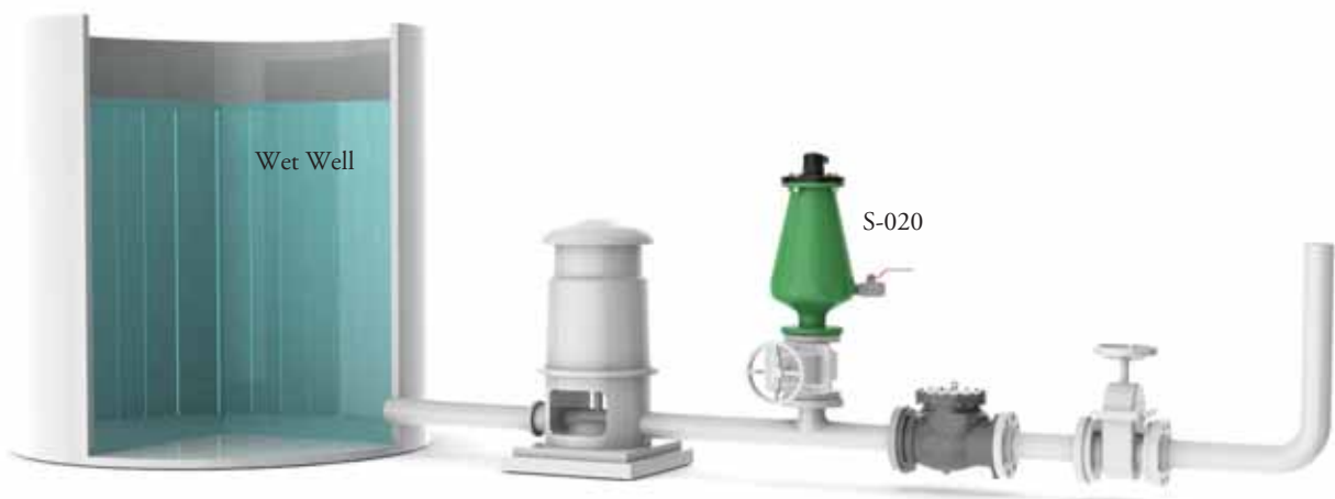
Dry well pumping.
