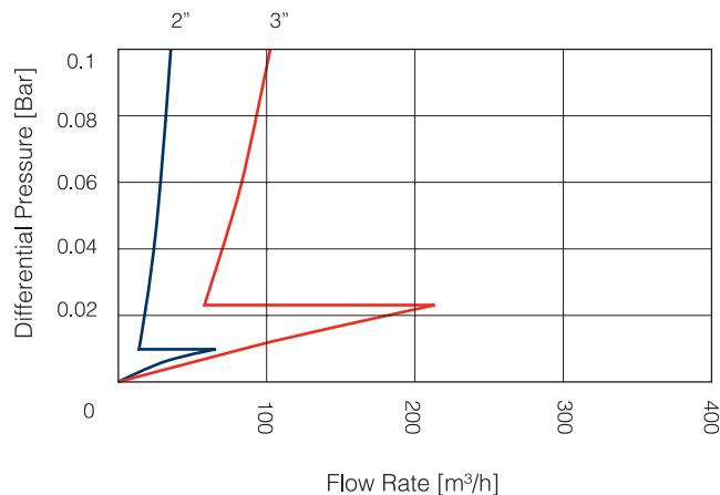
PN 16 AUTOMATIC AIR RELEASE FLOW RATE
