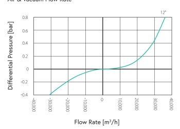
Automatic Air Release Flow Rate
