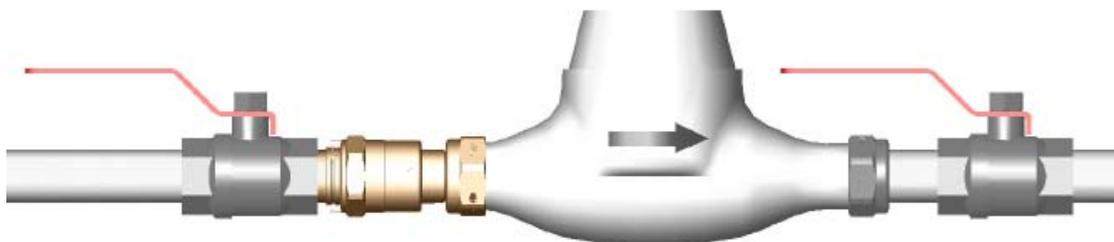
Figure 2 – Connection of UFR with union nut connection, upstream of the water meter.
