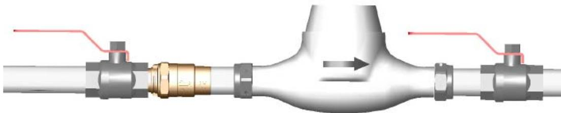
Figure 4 – Connection of **UFR** with threaded male or female connections, upstream of the water meter directly to the shut off valve and water meter coupling.
