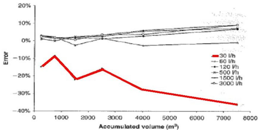
**Figure 2:** Multi-jet error (nominal flow  $1.5 \text{ m}^3/\text{hr}$ ) on accumulated volume (Arregui et. 2006, p.21)
