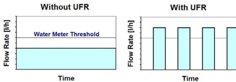
**Figure 7:** UFR – Principle of Operation
